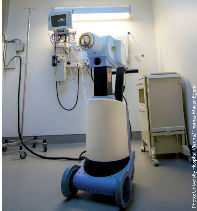
Various devices are used in brachytherapy, such as an afterloader shown here.
